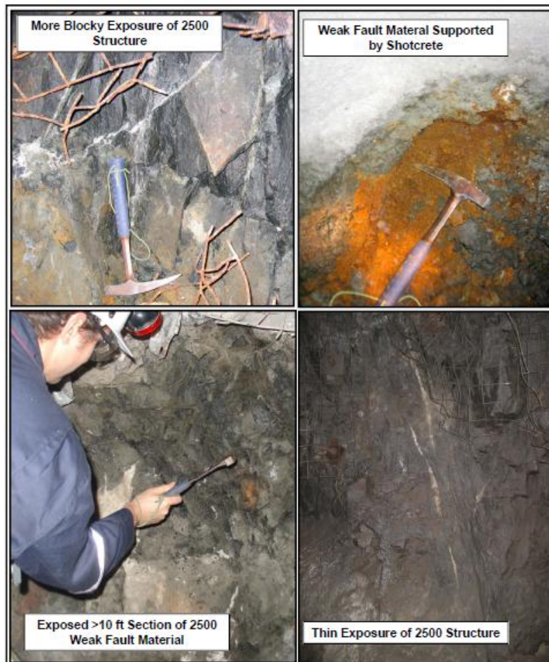
Figure 4: Fault material characteristic variation, as observed at different locations along the same fault .
