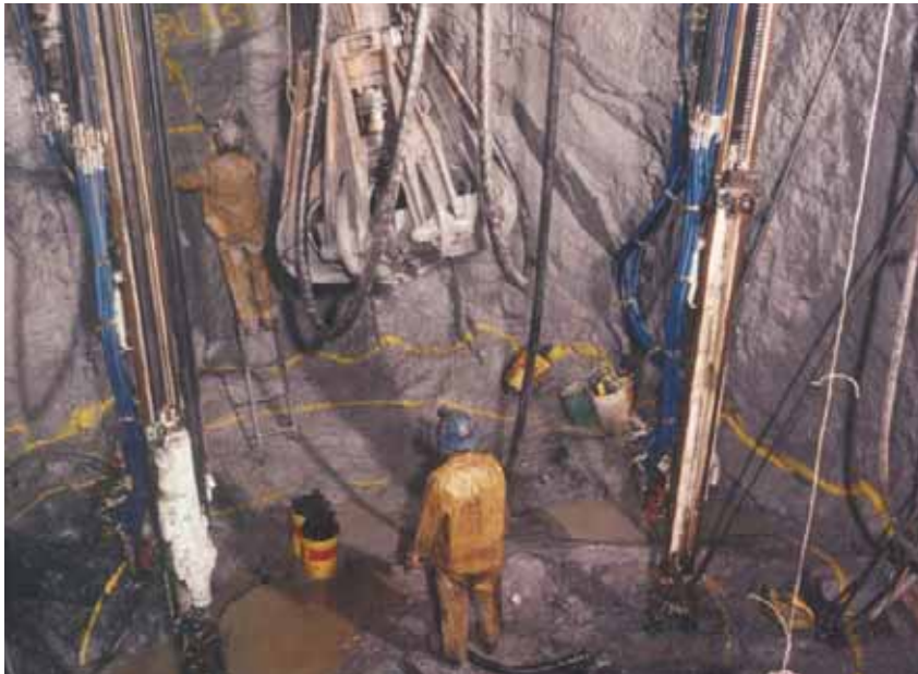
In addition to manufacturing a wide line of underground loading and haulage equipment, Sudbury, Ontario-based MTI also produces tunneling and shaft-sinking equipment such as the shaft jumbo rigs shown here.
